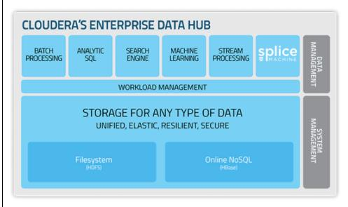
Using HBase as its storage layer, Splice Machine natively runs in the Hadoop stack, ensuring smooth integration to the ecosystem of Hadoop tools, such as Yarn, Hive, Spark, ZooKeeper, Flume, Storm, Kafka, and Sqoop. Using HBase co-processors, Splice Machine can efficiently execute complex SQL statements concurrently on parallel HBase nodes without the overhead of MapReduce.
